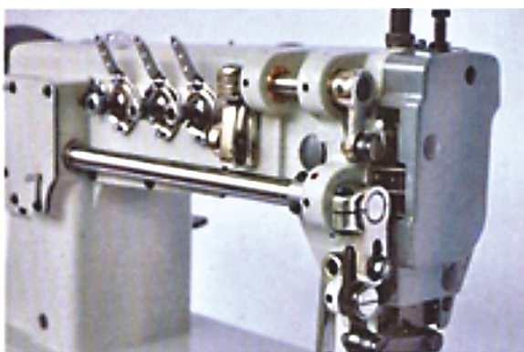
Back view showing linkage for the upper feed
