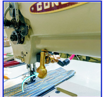
Clinton Knuckle Switch for convenient control of Air Reverse Function
