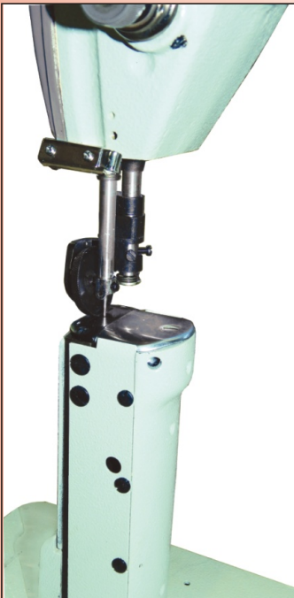
Closeup of 228R-11-1 needle and roller foot
