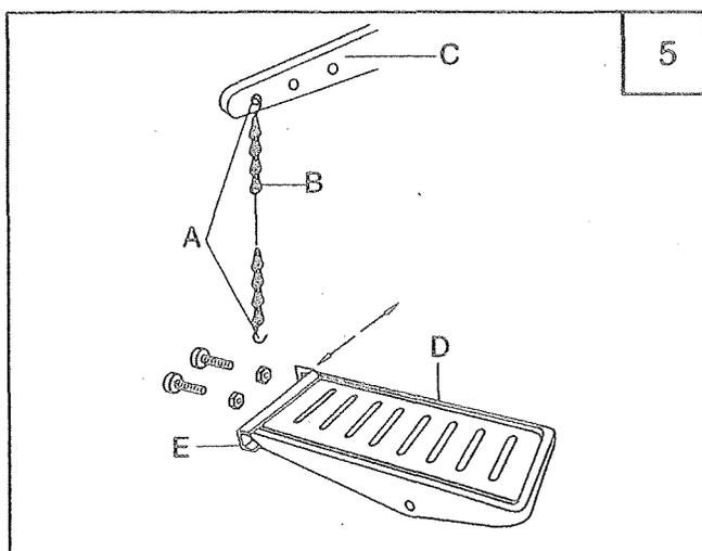
First, the chain hook A should be connected to the presser foot lift lever C, then put the pedal assembly D on the stand, move the control plate E leftward or rightward until the chain becomes on one line, Tighten the bolts and nuts, finally, connect the chain hook to the control plate.
