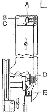
The bobbin thread should be neat and tight. If the thread is weak, please increase the tension of the thread tension disc A; if the thread is not neat, please move the bracket C to adjust it. First, loosen the screw B, if the thread is wound to one side as Fig ②, move the bracket rightward; if it is as Fig ③, please move the bracket leftward until the thread is wound neatly as Fig. ①, then tighten the screw.
