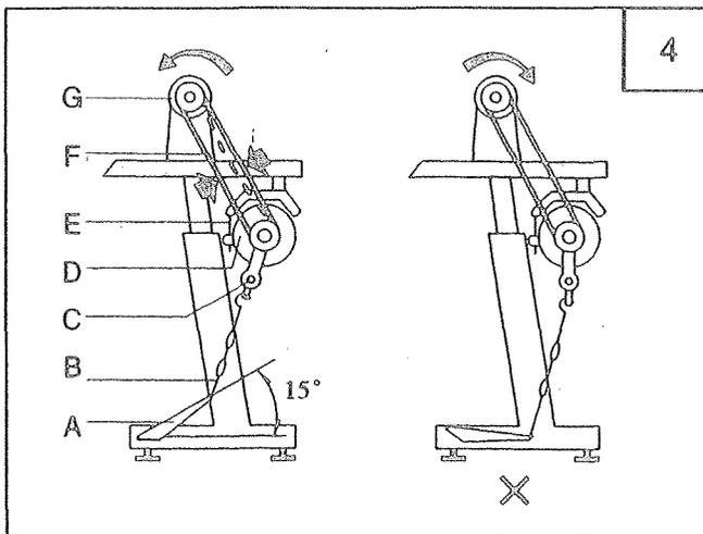
1. The optimum tilt angle of pedal A against floor is approx. 15° .
