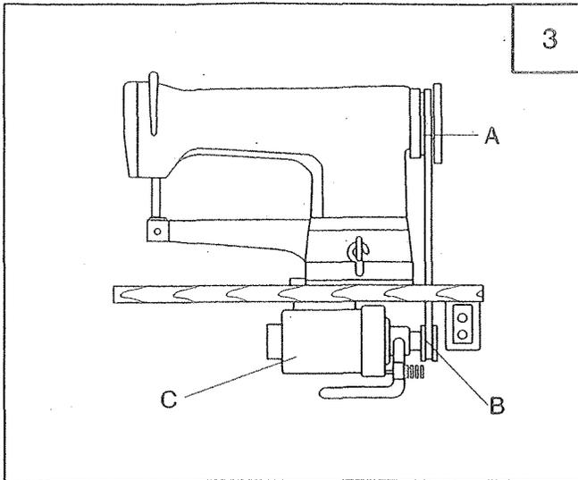
Align machine balance wheel belt groove A with motor pulley belt groove B by moving motor C leftward or rightward. Be sure that the belt is not touched with the table.
