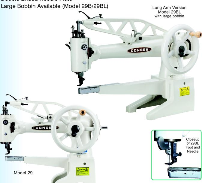
SINGLE NEEDLE 12" or 18" CYLINDER ARM SHOE REPAIR AND MENDING LOCKSTITCH MACHINE
