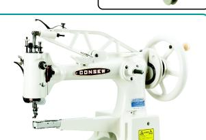
All 29's can have the hand wheel mounted on the **end**, as above, or on the **front**, as in the photos on the first page.
