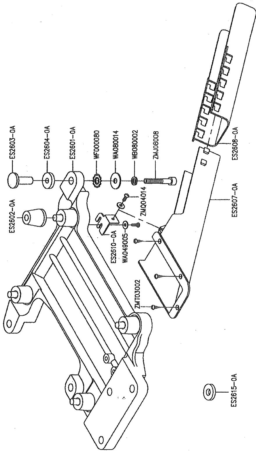
P. PARTS FOR SEMI - SUBMERGED INSTALLATION
