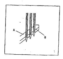
Front/Rear position of Needle Guard (Rear). When the tip of Looper comes to the center of right needle, adjust the clearance between Needle and Looper to 0-0.05mm by pressing Needle Guard (Rear). At this time, provide a clearance of 0-0.05mm between left needle and Needle Guard (Rear). These adjustments are made by 100sening Screw (R) and (C).
