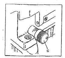
When using the Differential Feed Control Lever, fix it at the desired position with Nut (E) within the range from the position of graduation On Lever when turning Knob(C) to Stopper (D) At the time of using max differential feed, turn Knob(C) and set Lever at 1. To adjust feed amount during operation, attach a chain to the Lever. (The range of differential ratio varies according to the stitch length. Refer to the table below.
