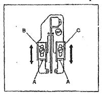
When using heavy wool thread, move Thread Eyelet (B) and (C) all the way forward so the thread does not pass between Supplementary Tension Discs (D).
