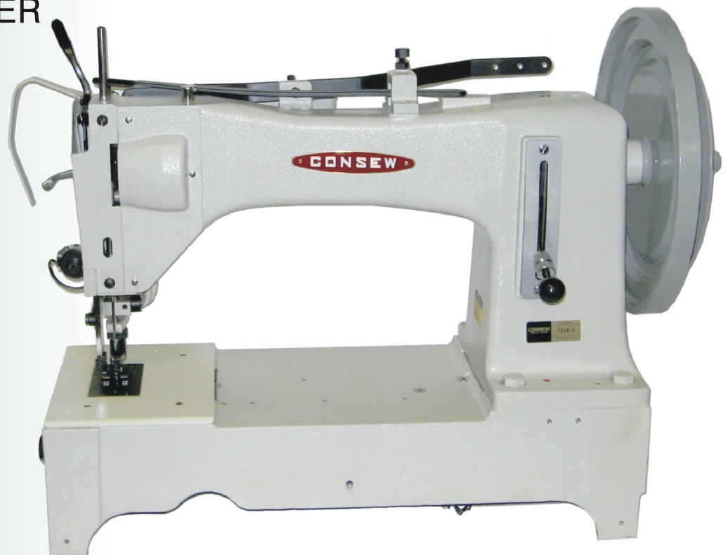
Detail of 733R-5 showing the two row feeder and the 1-1/4" extra high foot lift
