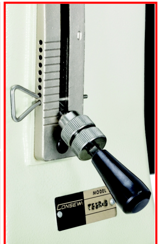
Stitch Length Lever with non-slip pin
