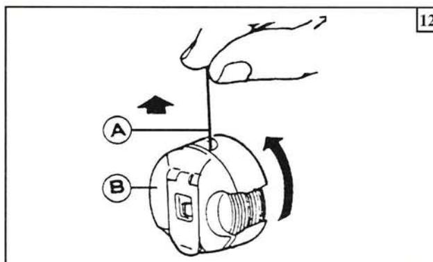
adjusted by changing tension of the thread take-up spring sewing range of the thread take-up spring tension of tension disc. and the position of thread guide.
