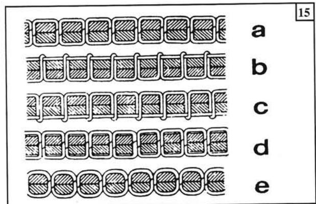
The position of the thread guide affects sewing quality so it must be adjusted according to the materials to be sewn.
