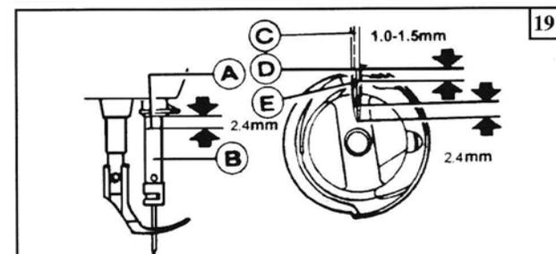
The motive relation between rotating hook and needle affects the sewing quality. Standard timing relation is: turn the balance wheel to locate needle bar to its lowest position, and loft back 2.4mm the rotating hook point (D) should be coincides with needle center line (C), and hook point (D) is 1.2mm above the upper edge (E) of needle eye.
