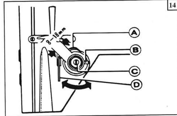
by 1/2 turn. After adjustment, tighten tension stud set screw (A).
