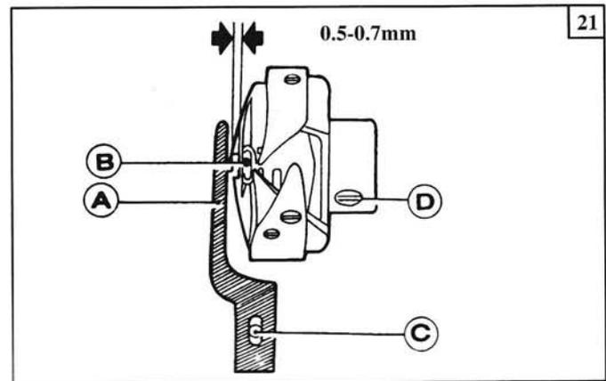
The projecting flange of the position bracket (A) should be engaged in the notch(B)of the bobbin case holder, and maintain a clearance of 0.5~0.7mm between projecting flange top and the bottom of notch while installing.
