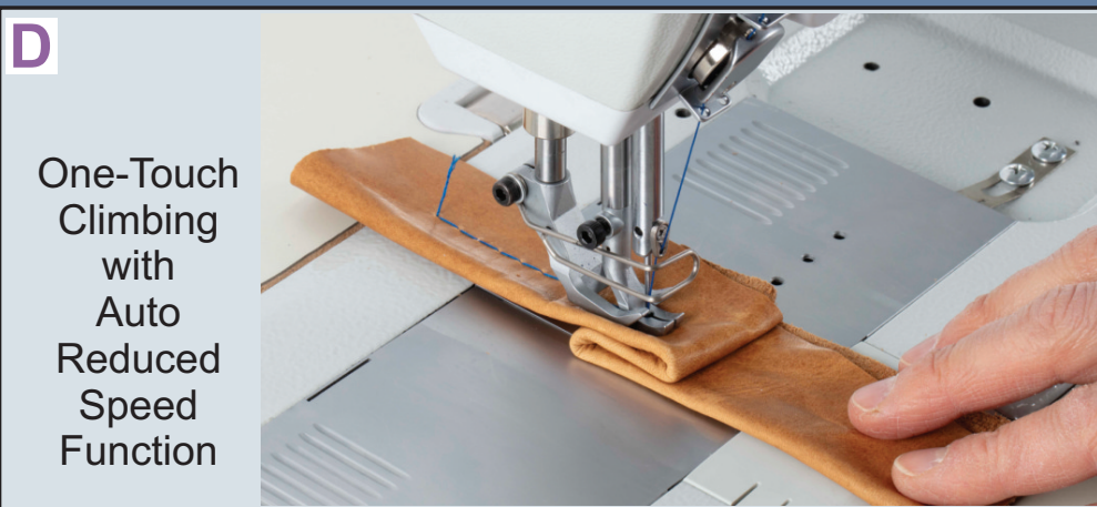
1-button automatic switching between different stitch lengths
