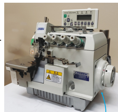
CM795-7DD showing location of the built-in motor
