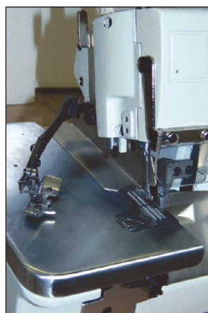
Detail of CM795 showing convenient swing-out presser foot assembly
