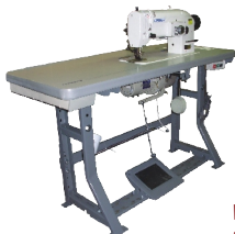
Example of sewing machine installed in a K-Leg Stand
