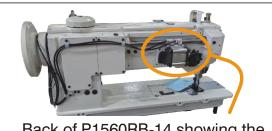
Back of P1560RB-14 showing the Footlift Air Lines and Air Cylinder.
