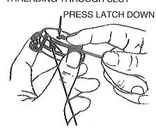
THREAD PULLED DOWN THROUGH SLOT
