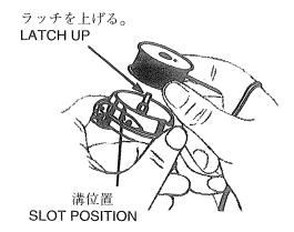
Replacing Bobbin in Case
