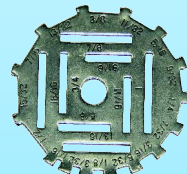
UMD Stitch Length measuring Tool
